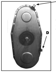
**Every 250 hours or Annually:** Change the gearbox oil. This operation performed at least once a year. Check the level of the transmission lubricant by removing bolt **D**, if necessary add EP1 grease after removing the cap **F**.
