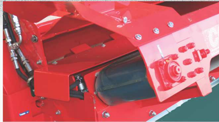
Robusto nastro in gomma rinforzata Heavy duty rubber conveyor belt
