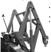
Attach the hitch to the machines via pins A and B
