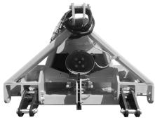
On **Folding** models move the brackets between the appropriate plates to match your tractor linkage category
