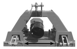
Adjusting the lower linkage on **Rigid** models is very simple: Remove the pins and swap the brackets from left to right.
