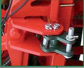
Attacchi flottanti Floating linkage Attelages Flottants Pendelnde Anhängunge
