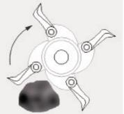
To replace the blades machine must be lifted and the blades replaced from underneath, make sure the machine is properly supported and made safe. Belt tension observation slot
