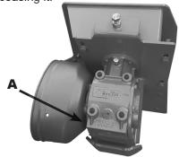
To control the oil level in the gearbox use tap **A** located behind the plastic guard. The guard must be removed in order to access tap **A**.
