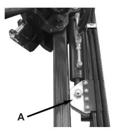
Depending on the tractor linkage and PTO position, when the DS-SS-MS are fully side shifted there is the possibility that the PTO shaft interferes with parts on the machine and could get damaged. It is important to adjust the amount of side travel in order to avoid damages and malfunctions.
