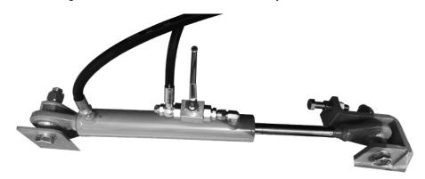
The tap on the machine ram must be opened during use and closed during transport. This acts as a safety block, restricting oil flow and therefor locking the implement in its position. During transportation the mower should never be in the upright position.
