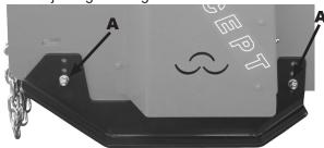
A The roller in the GTS is an integrated part of the rear tailgate. To alter the height of the skids remove bolts A, reposition the skid in the desired height and fasten bolts A.
