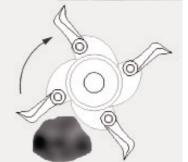
Check the bolts for tightness and the flails for wear and breakages. Replace all broken, bent or worn blades.
