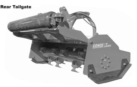
The rear roller is incorporated in the tailgate which can be opened via hydraulic rams. Opening the tailgate allows the user to reverse on to large piles of prune cuttings, debris from forestry work and shrubs bushes and trees up to 15 cm in diameter.
