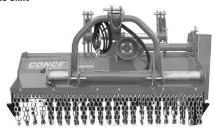
The hydraulic side shift is very simple and requires very little maintenance, simply connect the hoses to the tractors double acting spool valve. Make sure there are no oil leeks and that the side shift tube is well lubricated. Grease the grease nipple provided every 10 working hours to reduce wear.
