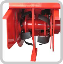
Each segment is enclosed by rotating divides which cut through the ground separating the cultivated row from the non-cultivated row.
